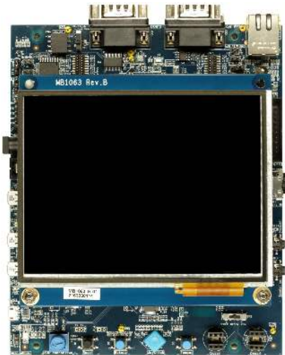
STM32H743I-EVAL and STM32H753I-EVAL top view. Picture is not contractual.
