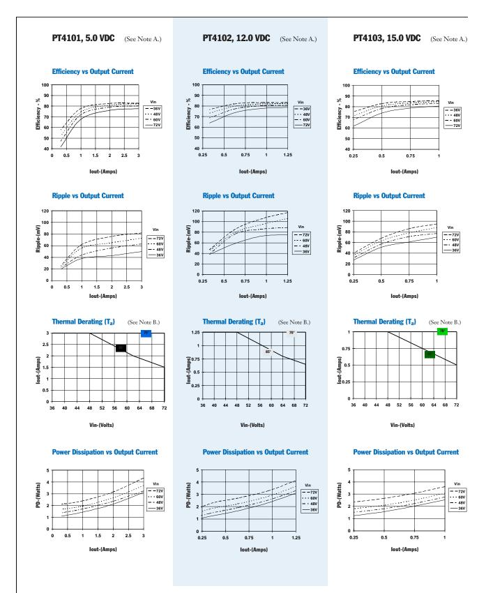
Note A: All data listed in the above graphs, except for derating data, has been developed from actual products tested at 25°C. This data is considered typical data for the DC-DC Converter. Note B: Thermal derating graphs are developed in free air convection cooling of 40-60 LFM.
