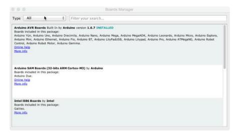
Next, quit and reopen the Arduino IDE to ensure that all of the boards are properly installed. You should now be able to select and upload to the new boards listed in the Tools->Board menu.
