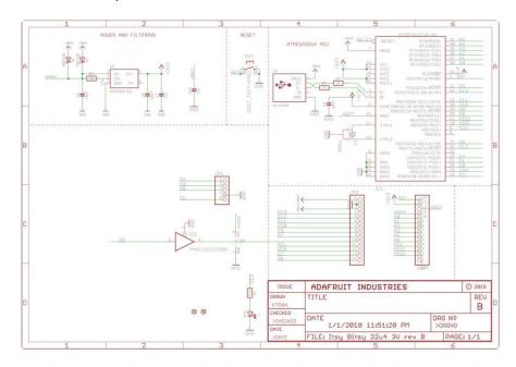
The 3.3V schematic regulator should be AP2112K-3.3
