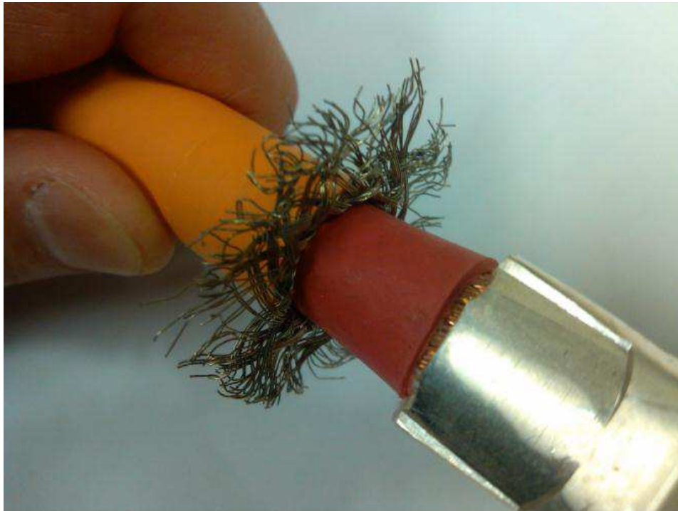
Figure 5: Hackle the shield braid
