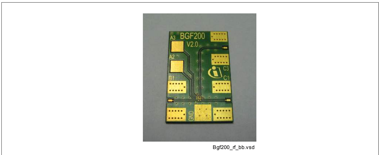
Figure 3 Bare RF Board
