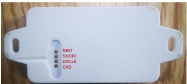
Use a metal wire to short NRST and GND pin will reset the LHT65.
