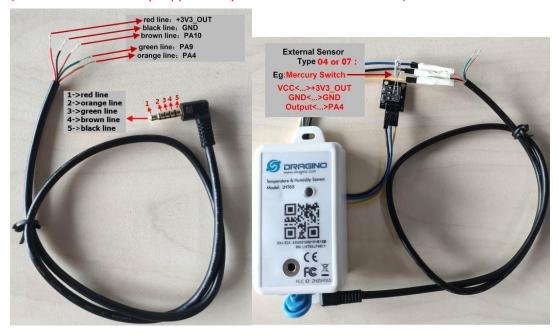
Above is connection to a mercury switch, rotate the mercury will generate interrupt. LHT65 will detect it and send an uplink package to sever. User can also connect PA9 and PA10 together, with these two pins shortcut, LHT65 will know if the probe is connected well in the socket.
