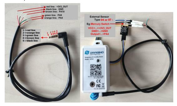
Above is connection to a mercury switch, rotate the mercury will generate interrupt. LHT65 will count it. It will periodically the counting value to server. User can also connect PA9 and
