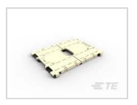
IC Socket Type: LGA 3647 Connector System: Board-to-Board Number of Positions: 3647 Contact Mating Area Plating Material Thickness: [30 µin] Centerline (Pitch): .86 mm, .99 mm [.034 in, .039 in]
