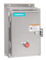
Non-reversing motor starter, Size 1, Three phase full voltage, Solid-state overload relay, OLR amp range 0.25-1A, 110V 50Hz / 120V 60Hz coil, Non-combination type, Encl. type 4X 304 S. Steel, Water/dust tight noncorrosive, Standard width enclosure
