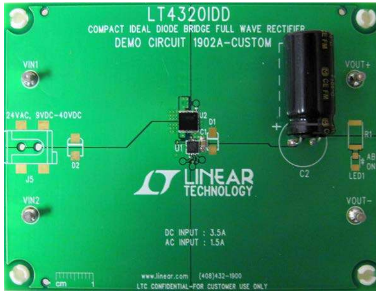
Figure 4. Demonstration Circuit 1902A Used in Figure 3 Thermograph
