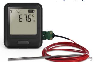
Lascar now offers a Traceable Calibration Certificate Service on Temperature Data Loggers. Using reference equipment which has been calibrated by a UKAS/NIST accredited laboratory and using apparatus traceable to national or international standards. For more information please see www.lascarelectronics.com.
