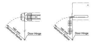
When the door hinged is on the extension line of the actuator mounting surface:
