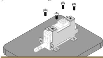
2pcs of M3.0 x 8 Bolts are for Bracket plate. Apply 4pcs of proper M3.0 screws at your end according to your condition.
