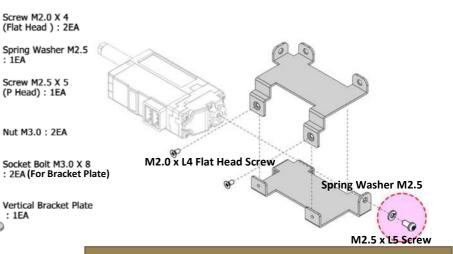
Make sure to use M2.5 spring washer to prevent damage.
