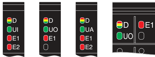
Figure 2-2 D and E LEDs on the power connectors of the I/O modules (examples)
