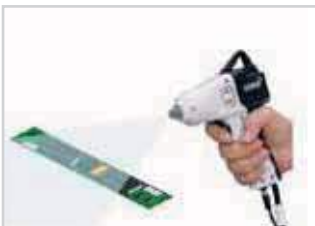
Remove dust on PCB
