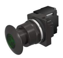
30mm BlackMax, Epoxy Coated Corrosion Resistant Complete Metal Unit Illuminated Push-Pull Operator Transformer type, 120V AC Incandescent Lamp Mushroom Head Cap Small 1 3/4" (44.5 mm) Metal, Black with Green Lens 2 Position Maintained, Pull-to-Release UL Listed, CSA Certified NEMA 1,3,3R,4,4X,12,13 & Automotive Standards
