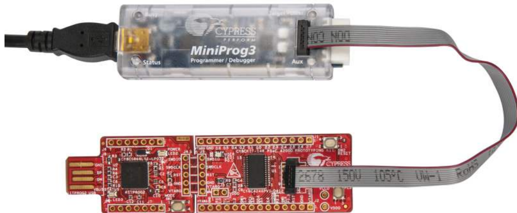
Figure A-16. Connecting the CY8CKIT-146 to a MiniProg3
