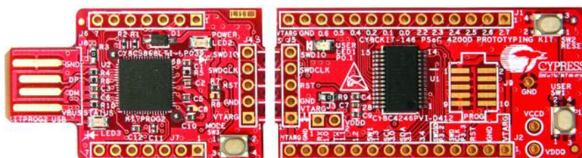
Figure A-4. PSoC 4200DS Prototyping kit Broken into Two Parts
