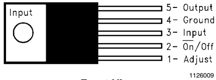
Front View TO-220, 5-Lead, Straight See NS Package Number T05A
