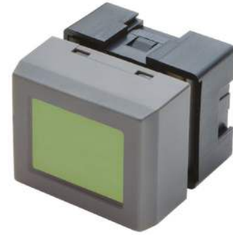
Red/Green Bicolor LED with Yellow LCD Mode
