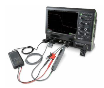
CP030 30A current probe and HVD3106 high voltage differential probe connected to an HD06104A-MS 12-bit resolution high definition oscilloscope. The DCS025 is connected to the EXT input (to conserve analog channels) and the deskew amount is adjusted for one of the probes in the channel dialog menu.
