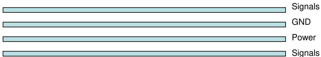
Figure 21: Typical 4-layer PCB construction
