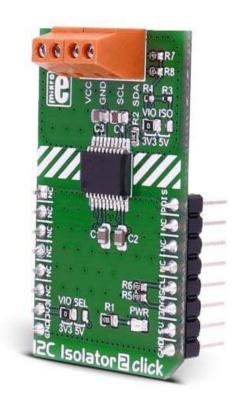
**I2C Isolator 2 click** provides I2C lines and power isolation for slave devices. It carries the ADM3260 dual I2C isolator with an integrated DC-to-DC converter. I2C Isolator 2 click is designed to run on either 3.3V or 5V power supply. The click communicates with the target microcontroller over an I2C interface with additional functionality provided by the PWM pin on the mikroBUS™ line.
