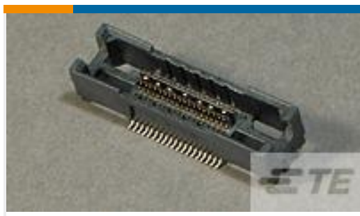
TE Part #2-5767004-2 MICTOR RECEPT ASSY, 38 POS.
