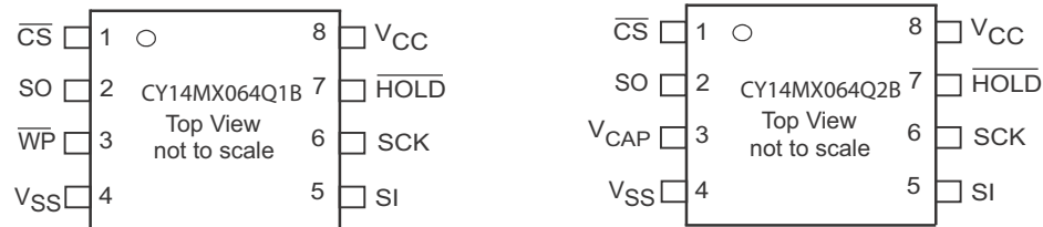
Figure 1. 8-pin SOIC pinout [1, 2]
