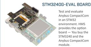
Test and evaluate Anybus CompactCom in an STM32 environment. HMS provides the option board — You buy the STM3240 and the Anybus CompactCom module.
