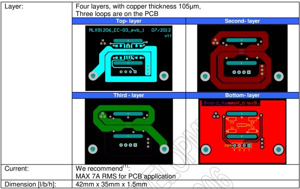
(1): The maximum current is limited by the PCB. For higher currents (> 10A), one can use EC-01, EC-02 or an external conductor (i.e. a bus bar).
