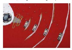
Continue this trace down and around to the negative pin of the Arduino. I neglected to get a picture of this connection, but just be careful not to touch the other traces and to pin it down well with several stitches. Next, cut and knot your thread, and get ready for the final trace! Sew down the positive pin on the buzzer.
