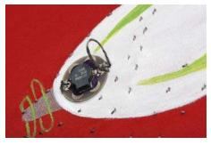
Flip over the circuit to the back side. You can see the two traces between the LEDs and pins 5 and 6, which will need to be crossed. Cut a piece of felt or another thick fabric, or create an alternative bridge if you prefer- you just need something that will insulate between this trace and the previous ones.
