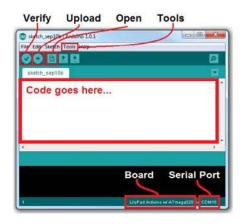
Before you can upload code, there are a few settings to make. Notice how in my picture above "Board" is correctly set as "LilyPad Arduino w/ ATmega328"? Yours is most likely not set that way. To change that, go to the **Tools** menu, navigate to the **Boards dropdown**, and select **LilyPad Arduino w/ ATmega328**. That tells the Arduino software what kind of board to compile code for.
