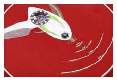
Sew down the positive side of the next LED, connecting it to pin 6.
