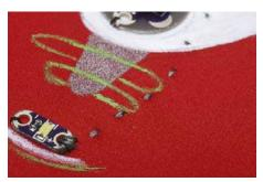
Sew from that positive hole to pin 5 of the Arduino board. You'll want to skirt around the buzzer a little ways, to leave room for the negative trace to leave the buzzer. When you get to pin 5, stitch it down several times before knotting and cutting your thread.
