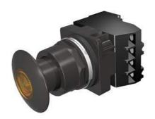
30mm BlackMax, Epoxy Coated Corrosion Resistant Complete Metal Unit Illuminated Push-Pull Operator Transformer type, 480V AC LED Lamp Mushroom Head Cap Small 1 3/4" (44.5 mm) Metal, Black with Amber Lens 2 Position Maintained, Pull-to-Release with 1 N.O. - 1 N.C. Heavy Duty Contacts, A600/P600 UL Listed, CSA Certified NEMA 1,3,3R,4,4X,12,13 & Automotive Standards
