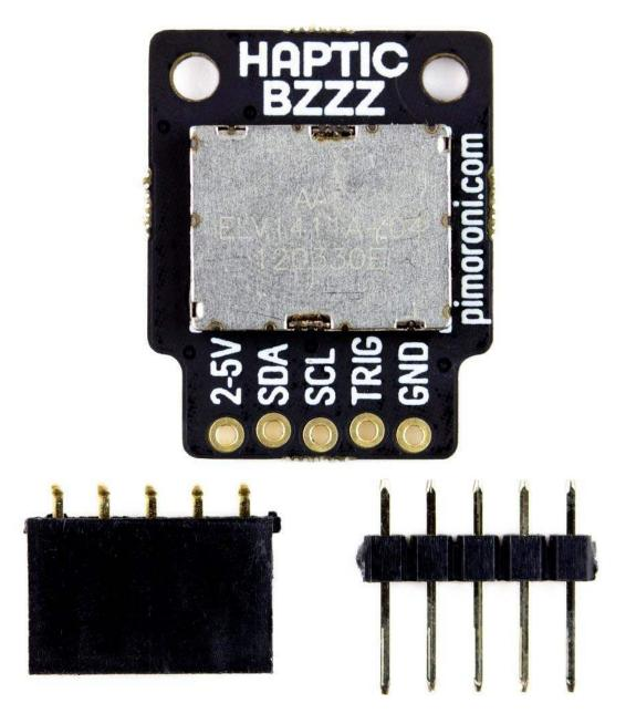
DRV2605L Linear Actuator Haptic Breakout PIM452
