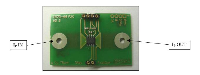
Connect then the primary between pins  $I_P$  IN and  $I_P$  OUT.
