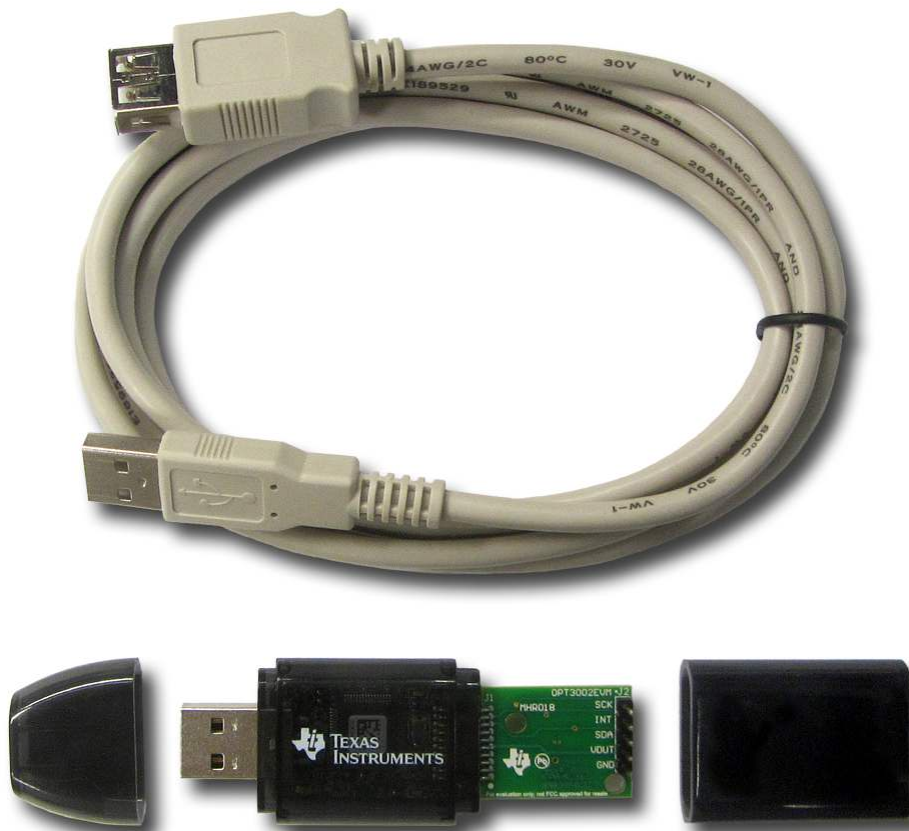
Figure 1. Hardware Included With OPT3002EVM Kit
