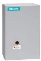
Non-reversing NEMA contactor, Size 3, Three phase full voltage, Contactor amp rating 90A, 3 wire (NO aux included), 24VAC 50-60Hz coil, Non-combination type, Enclosure NEMA type 1, Indoor general purpose use, Standard width enclosure
