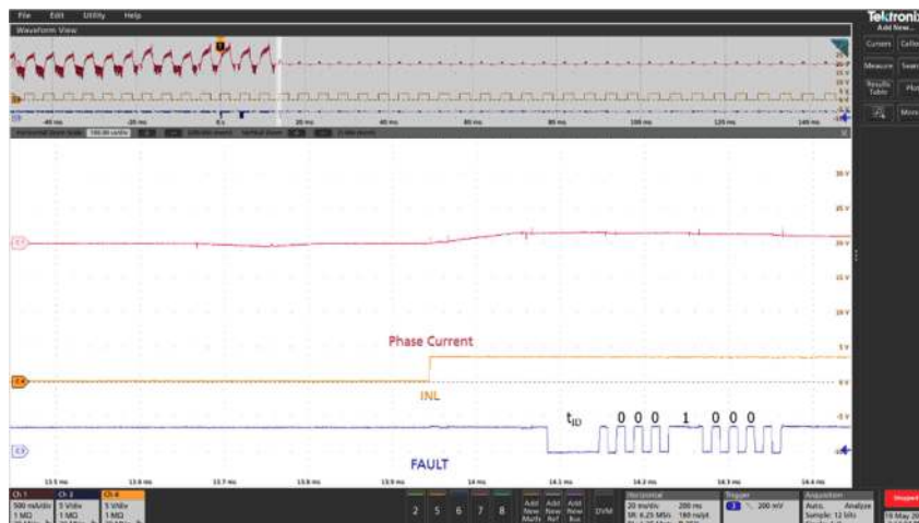
Figure 31 – CH1: I_{PHASE} , 500 mA / div. CH3: V_{INL} , 5 V / div. CH4: V_{INL} , 5 V / div. Time: 20 ms / div. Zoom: 100 \mu s / div. Over-Temperature Protection U1.
