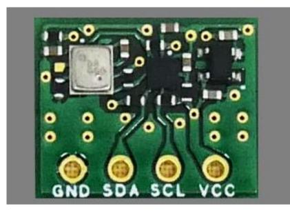
Barometric Pressure sensor device is capacitive type MEMS device combined with ASIC with I2C interface. Since its voltage level is 1.8V, there's level converter on this board, which enables user to connect directly to 3.3V system.
