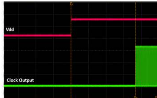
Figure 17. Startup Waveform vs. Vdd
