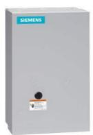
Non-reversing contactor, Size 2 1/2, Three phase full voltage, Contactor amp rating 60A, 3 wire (NO aux included), 110V 50Hz / 120V 60Hz coil, Non-combination type, Enclosure NEMA type 1, Indoor general purpose use, Extra-wide enclosure
