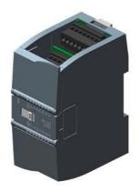
SIPLUS S7-1200 SM 1223 8DI/8DQ RLY based on 6ES7223-1PH32-0XB0 with conformal coating, -20...+60 °C, digital input/output 8 DI/8 DQ, 8 DI 24 V DC, sink/source, 8 DQ, relay 2 A
