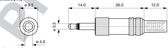
Cable diameter max. 4.0 mm
