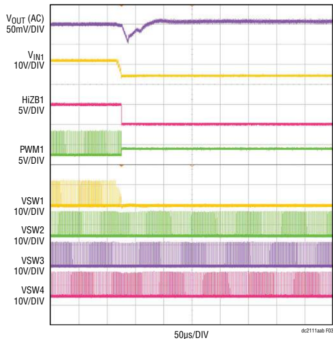
Figure 3. 1.2V/90A Converter with N+1 MOSFET Failure Protection. Bottom MOSFET of Phase 1 Shorted Drain to Source with Full Load on the Output and a 12V input. The Output Continues to Regulate with Only a Small Perturbation on the Output.
