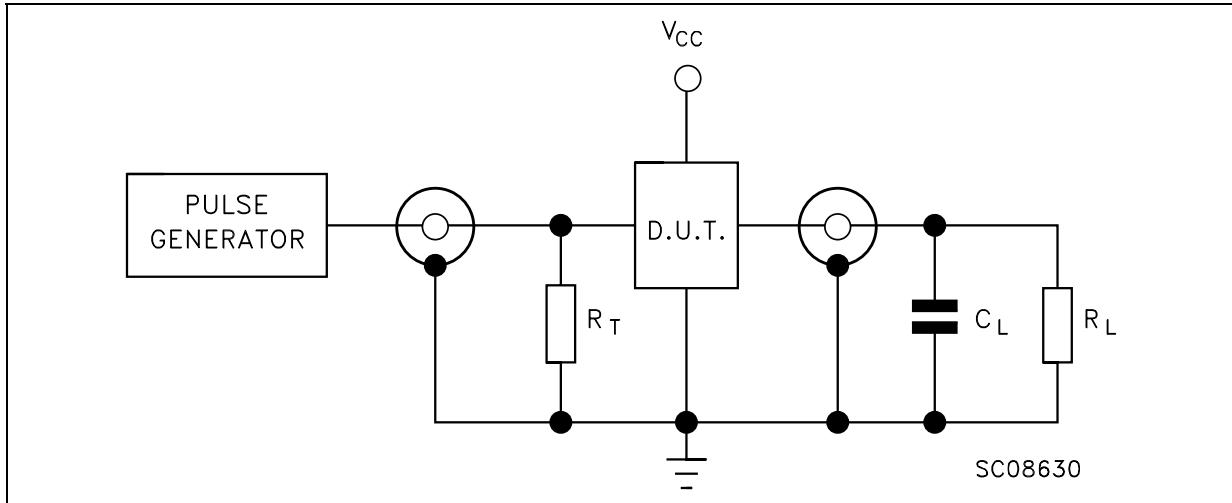
**TEST CIRCUIT AND WAVEFORM SYMBOL VALUE**
