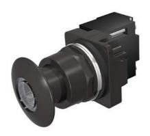
30mm BlackMax, Epoxy Coated Corrosion Resistant Complete Metal Unit Illuminated Push-Pull Operator Transformer type, 600V AC LED Lamp Mushroom Head Cap Small 1 3/4" (44.5 mm) Metal, Black with Clear Lens 2 Position Maintained, Pull-to-Release UL Listed, CSA Certified NEMA 1,3,3R,4,4X,12,13 & Automotive Standards
