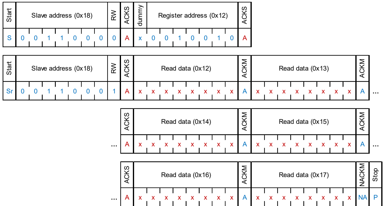
Figure 5: I 2 C multiple read
