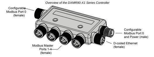
One male M12 connection provides common power and ground to all M12 Modbus ports. The two-port 0 Modbus connections can be configured as pass-through wiring to connect to a Modbus trunk. One 100 Mbps Ethernet port (female) using an M12 D-coded Ethernet connection.
