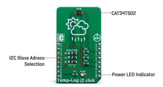
When set in the Interrupt Mode, the EVENT output will be asserted every time the temperature crosses one of the alarm limits. Once the temperature exceeds the critical limit, the EVENT remains asserted as long as the temperature stays above the critical limit. The EVENT can be cleared by setting a bit in a corresponding register (must be cleared by the software). However the pin will remain asserted as long as the temperature exceeds the critical limits.
