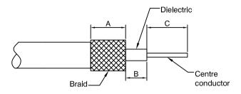
2) Insert the cable into the body. Ensure the inner mandrel is between the braid and the dielectric.
