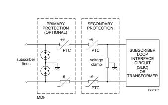
Fig.1 Typical telephone line equipment showing where PTC thermistors can be used for overcurrent protection.
