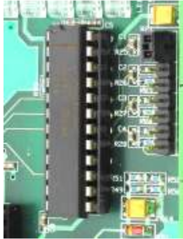
Figure 4: Oblique view of the 4-20mA Shunt Locations
