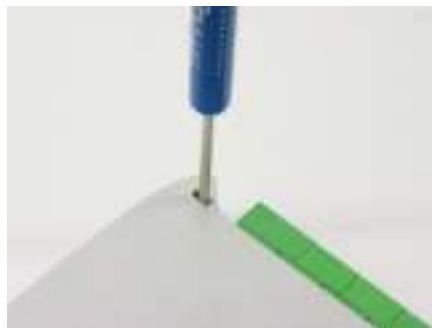
Figure 1: Opening the Stamp PLC Enclosure
