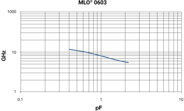
Typical Self Resonant Frequency vs. Capacitance MLO® 0603
