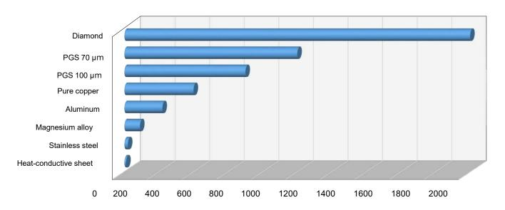
Coefficient of thermal conductivity W / (m·K)
