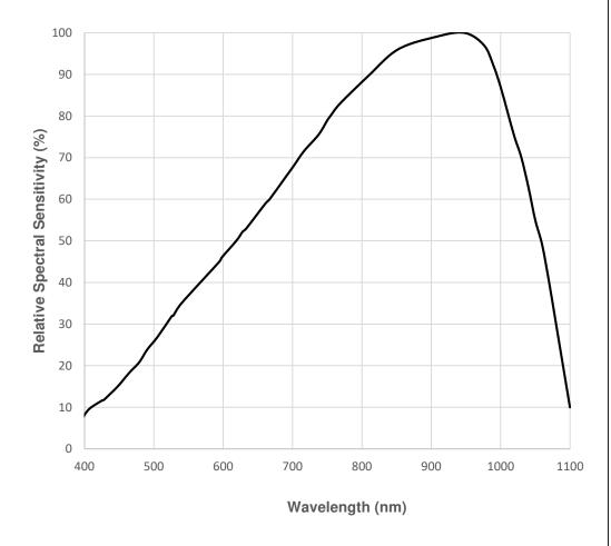
Testcondition:  $Ee = 0.5 \text{ mW/ cm}^2$ ; VCE = 5 V
