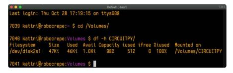
That's not very much space left! The next step is to show a list of the files currently on the CIRCUITPY drive, including the hidden files, using the ls command. You cannot use Finder to do this, you must do it via command line!
