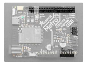
These are the logic pins that can be used to connect shields, sensors, servos, LEDs and more!
