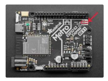
The Built-in Red LED is located in the upper right of the board below the OK LED and has the number 42 to the left of it.
