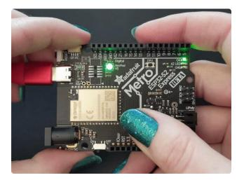
Before we upload a sketch, place your ESP32-S2/S3 board into ROM bootloader mode ().
