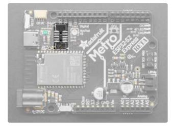
If you'd like to do more advanced development, trace-debugging, or not use the bootloader, we have the JTAG interface exposed. You'll need to solder an 2x5 1.27mm pitch connector () or Mini 2x5 connector () to your board. A JLink or similar is needed to perform debugging.
