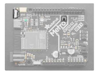
Reset button - The reset button in the top left corner is used to reset the board. DFU button - This is connected to BOOT0 and can be used to put the board into ROM bootloader mode. To enter ROM bootloader mode, hold down DFU button while clicking reset button mentioned above. When in the ROM bootloader, you can upload code and query the chip using esptool
