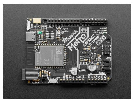
What's Metro shaped and has an ESP32-S2 WiFi module? What has a STEMMA QT connector for I2C devices, and a Lipoly charger circuit? That's right - its the Adafruit Metro ESP32-S2!
